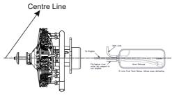
Note: Install the tank on the centre line of the engine
