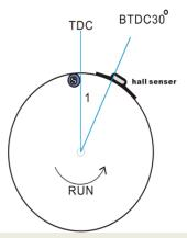
Bring engine to 30 Degree BTDC, The buzzer and Green LED should be coming ON when trailing edge of the sensor and magnet comes together. The ignition module should spark or if you use a timing device then correct set is when buzzer and/or Green LED turns OFF !!! And that is when magnet leaves the sensor
