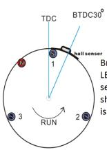
**Multi Cylinder Timing Set-up** 2 cyl "V", Boxer, Inline' 3,5,7,9 Radial Engines
